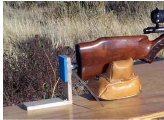
Rifle set up for making recoil measurements.
