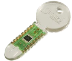
Demo Key molded in clear plastic to show internal memory chip
